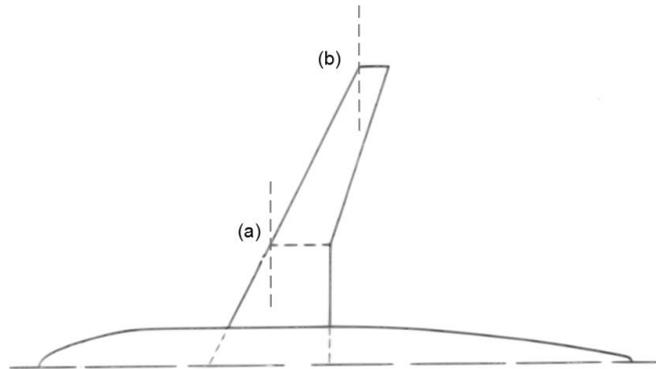
Figure 6 - Axes definition for twisting: (a) kink, (b) tip
