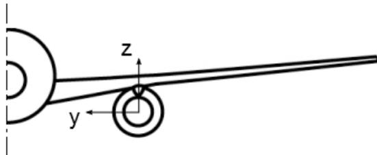
Figure 3 – Nacelle local axes
