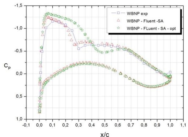
Figure 11 –  $C_p$  value near wing tip ( $\eta=0,847$ )
