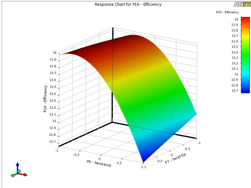
Figure 9 – Efficiency vs. twist kink and tip response surface
