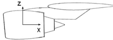
The presence and the position of the nacelle effects the aerodynamics of the wing and plays a role in the overall aircraft performance. The nacelle position is defined by three design variables: translation along z
