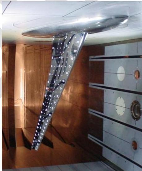
Figure 3. HIRENASD wind tunnel model
