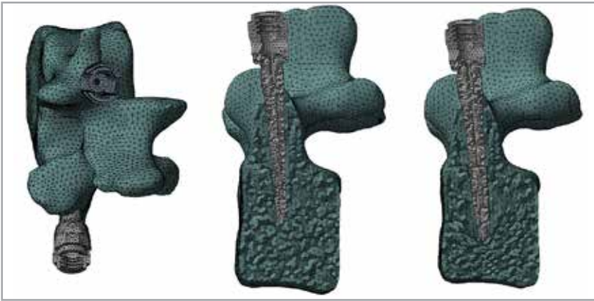
Fig. 15 – A patient-specific high-fidelity FEA model representing one vertebra and two prosthetic screws was created; mesh morphing allows the diameter and length of the screw to be updated to optimize individual patient treatment
