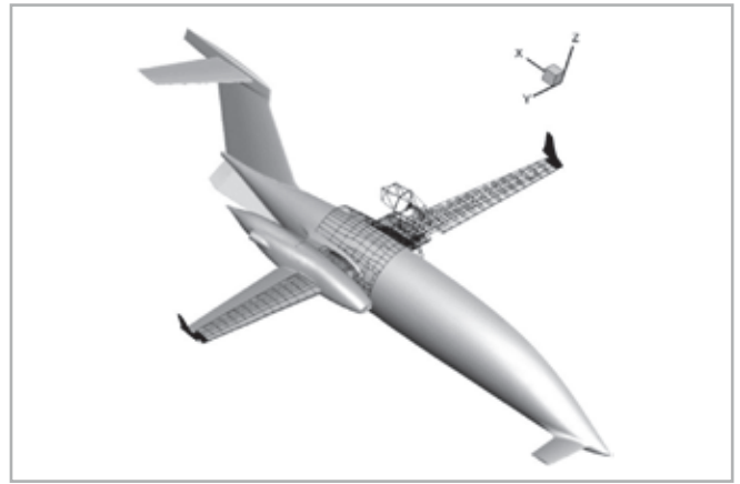
Fig. 4 - The CSM model and its position with respect to the CAD model
