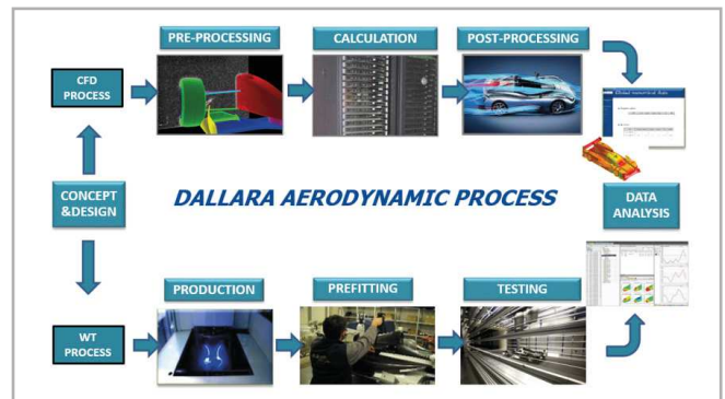
Fig. 3 – The aerodynamic process at Dallara: wind tunnel and CFD are combined to design and optimize aero shapes.
