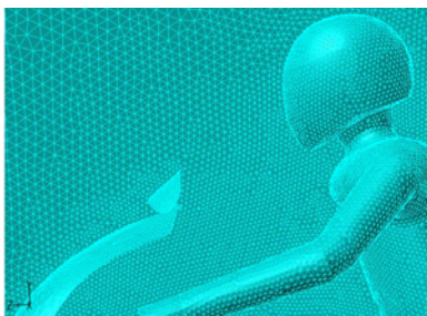
The mesh is morphed to vary driver angle between 0° baseline (left) and 15° (right), with respect to the vertical axis.
