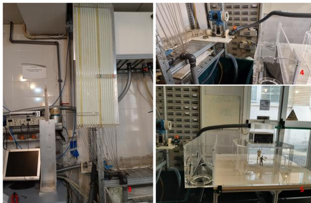
Figure 5.2.6: In the figure to the left is shown the pressure gauge; to the right at the top is shown the electromagnetic flowmeter, and at the bottom, the flowmeter that will be linked to the scale model.
