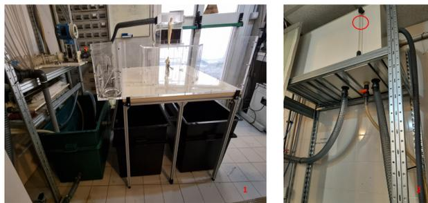
Figure 5.2.5: The figure shows to the left the scale model and three basins used to fill up the tank or to empty it, and to the right, the tank where is highlighted the maximum level of water called "overfull".
