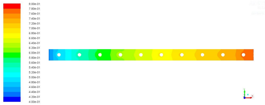
Figure 6.36: Overall effectiveness contour of plate in candidate point 1
