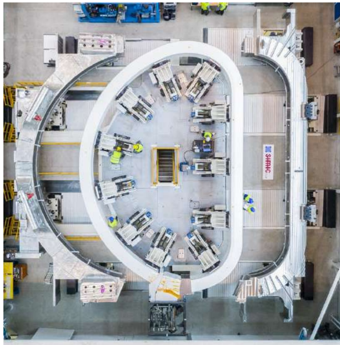
Figure 17: Coil Cases and WP assembly [37].
