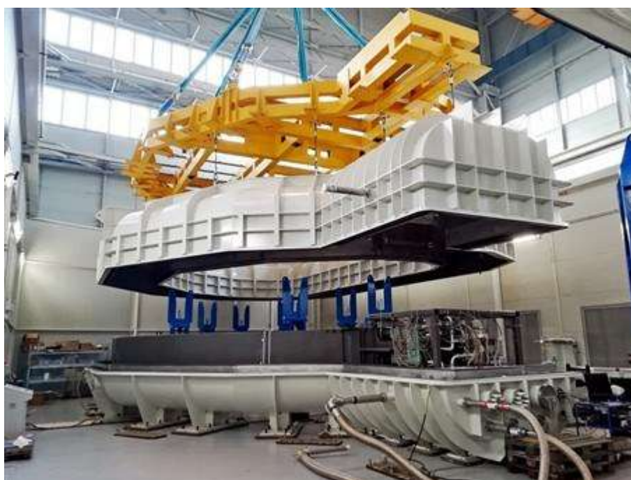
Figure 14: Winding Pack [Retrieved on 21 Jul 2022 on www.fusionforenergy.europa.eu ]
