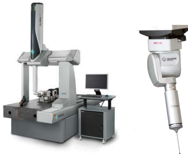
Figure 29: CMM machine [Retrieved on 21 Jul 2022 on www.hexagonmi.com ]
