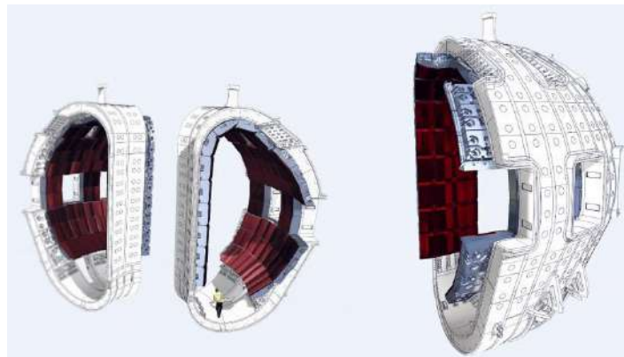
Figure 20: ITER Vacuum Vessel sector. [Retrieved on 21 Jul 2022 on www.iter.org ]
