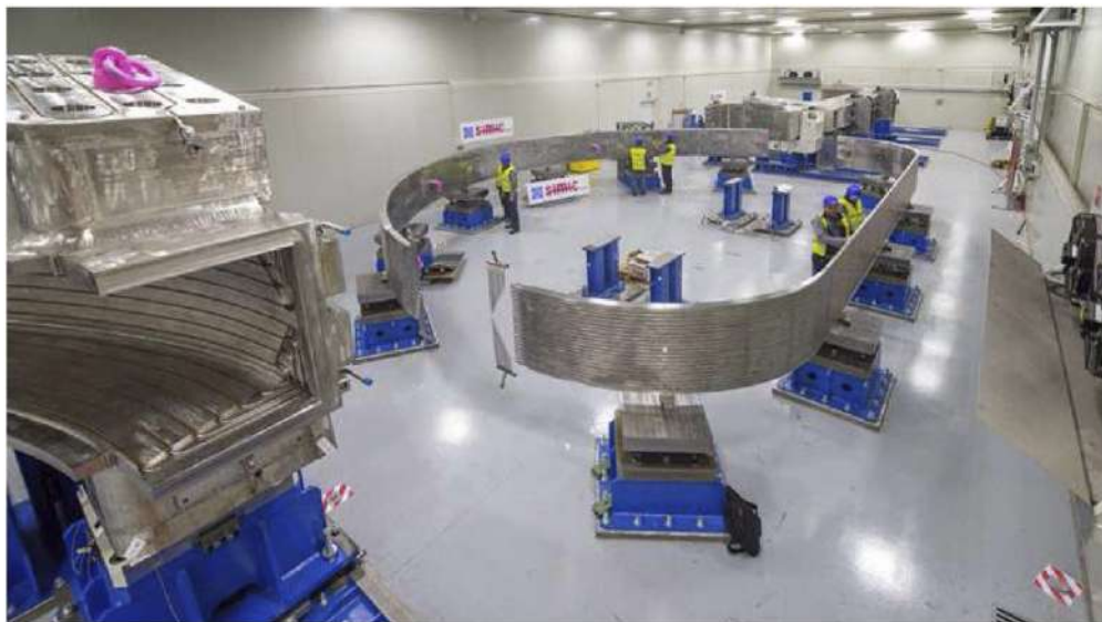
Figure 16: Coil Cases acceptance [37].
