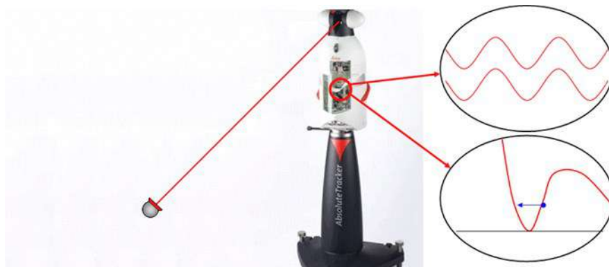
Figure 35: Absolute Laser Interferometer [Retrieved on 21 Jul 2022 on www.hexagonmi.com ]
