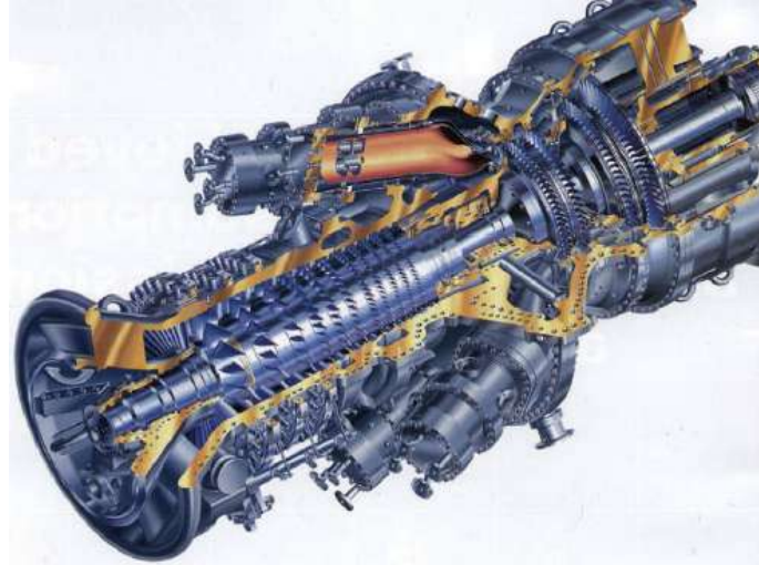
Figure 1.1: A frame-type gas turbine with DLE combustors.
