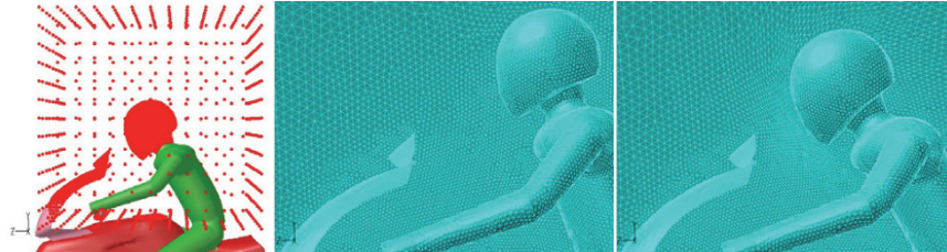
Fig. 1. Source points of an RBF problem and result of the mesh morphing action.
