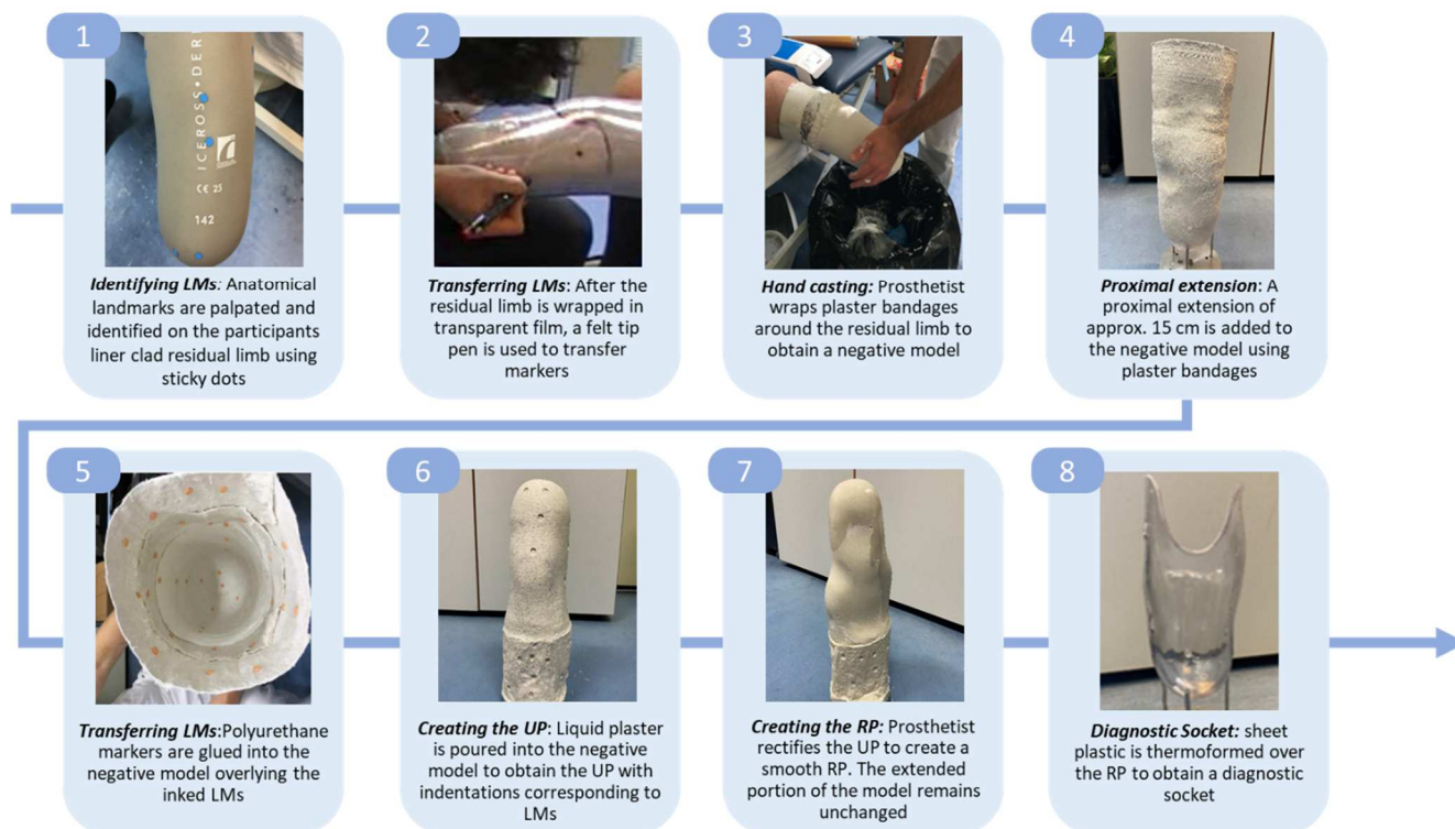
Figure 2. Schematic representation of the manual data collection required to create the training dataset (steps 1–7) and the final diagnostic socket fabricated to allow for the evaluation of the process (step 8). LMs: landmarks; UP: unrectified positive; RP: rectified positive.
