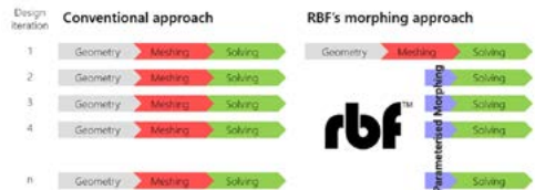
Figure 3: The automated workflow enabled by mesh morphing. New CAE variations are automatically generated making the baseline CAE model parametric. Design exploration and generation of synthetic big data to train reduced order model are substantially simplified with respect to the conventional approach based on parametric CAD and remeshing. The ability of generating shape variations with parameters (figure 3) allows to enable optimization according to zero-order methods (the shape parameters are used as input) and/or to local methods (steepest descent gradient when derivatives of KPI versus input parameters are available). The same
